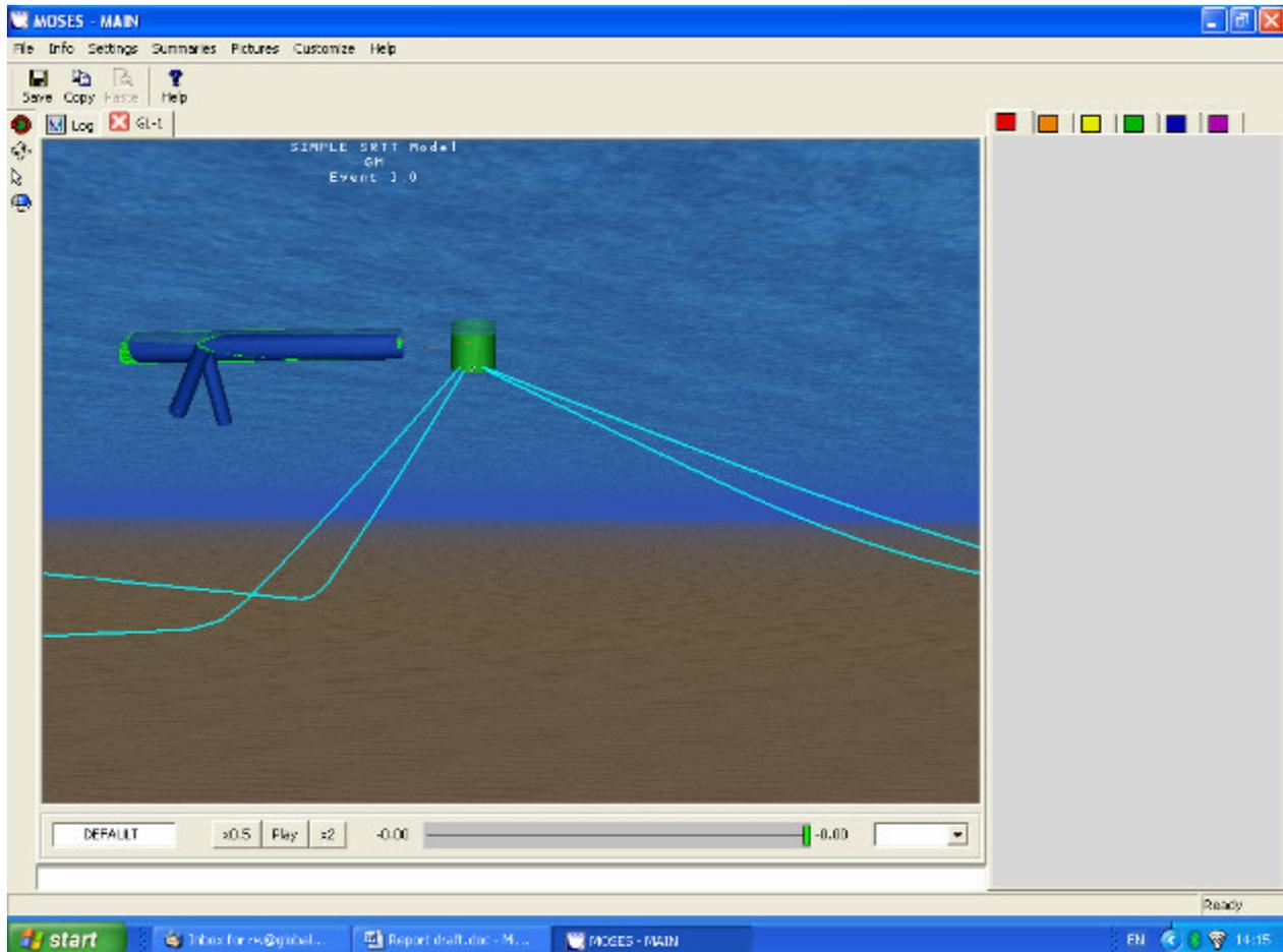
**Figure 3.1: 4-Point Mooring Arrangement**
