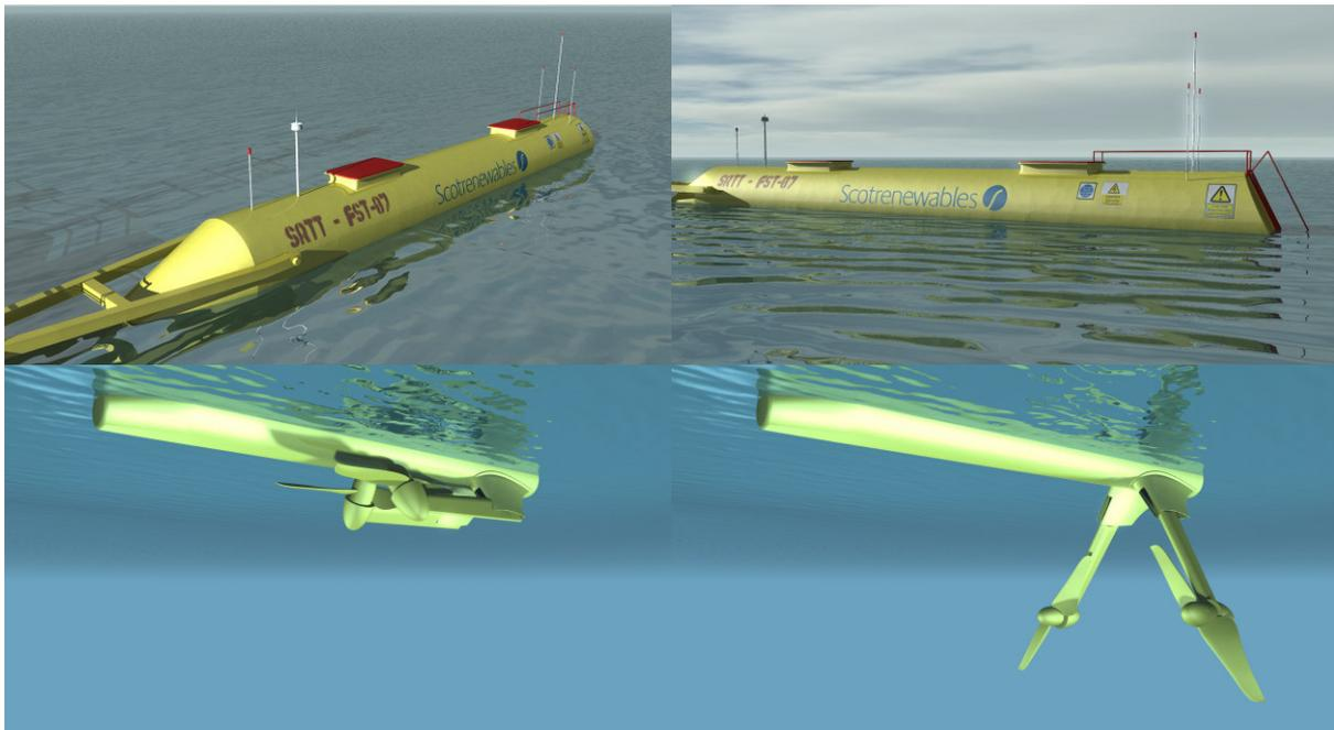
**Figure I: SRTT Transport and Operation Configurations**
