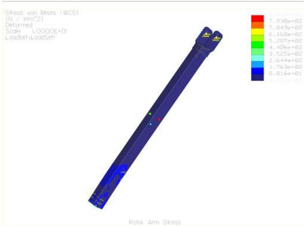
**Figure 2.10: Extreme Loading Stress Distribution**
