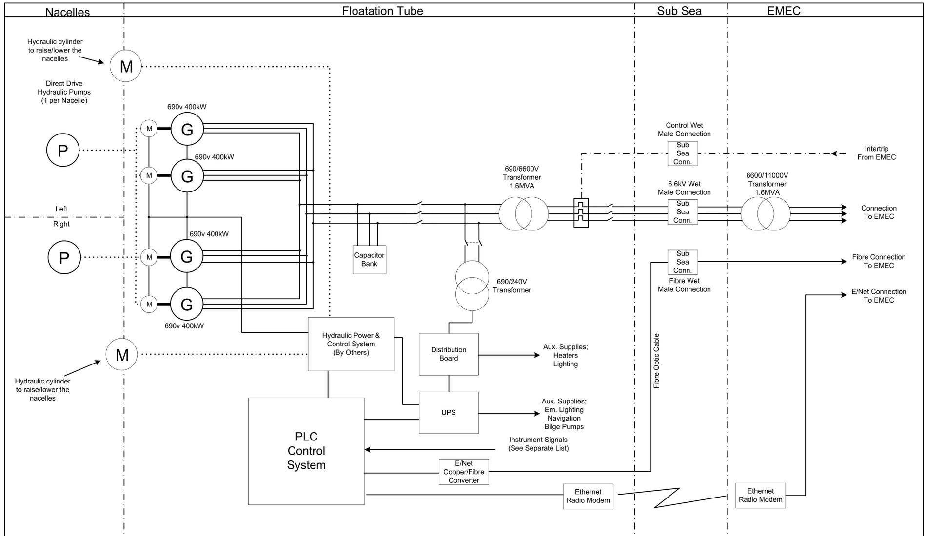
Figure 4.3: Hydraulic System with 4 Generators
