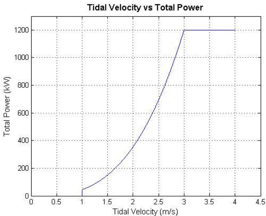
**Figure 2.2: Rated Power Curve for Static (No Wave) Conditions**
