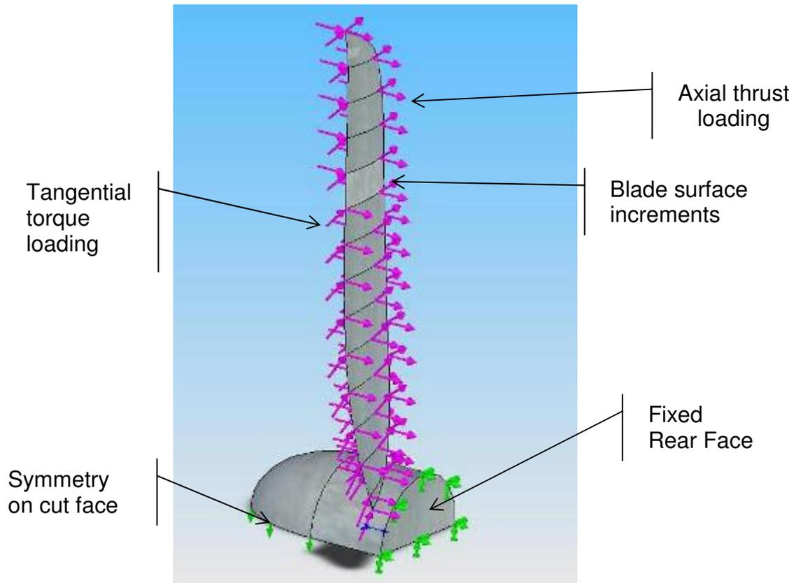
**Figure 2.8: Blade loading and boundary conditions**
