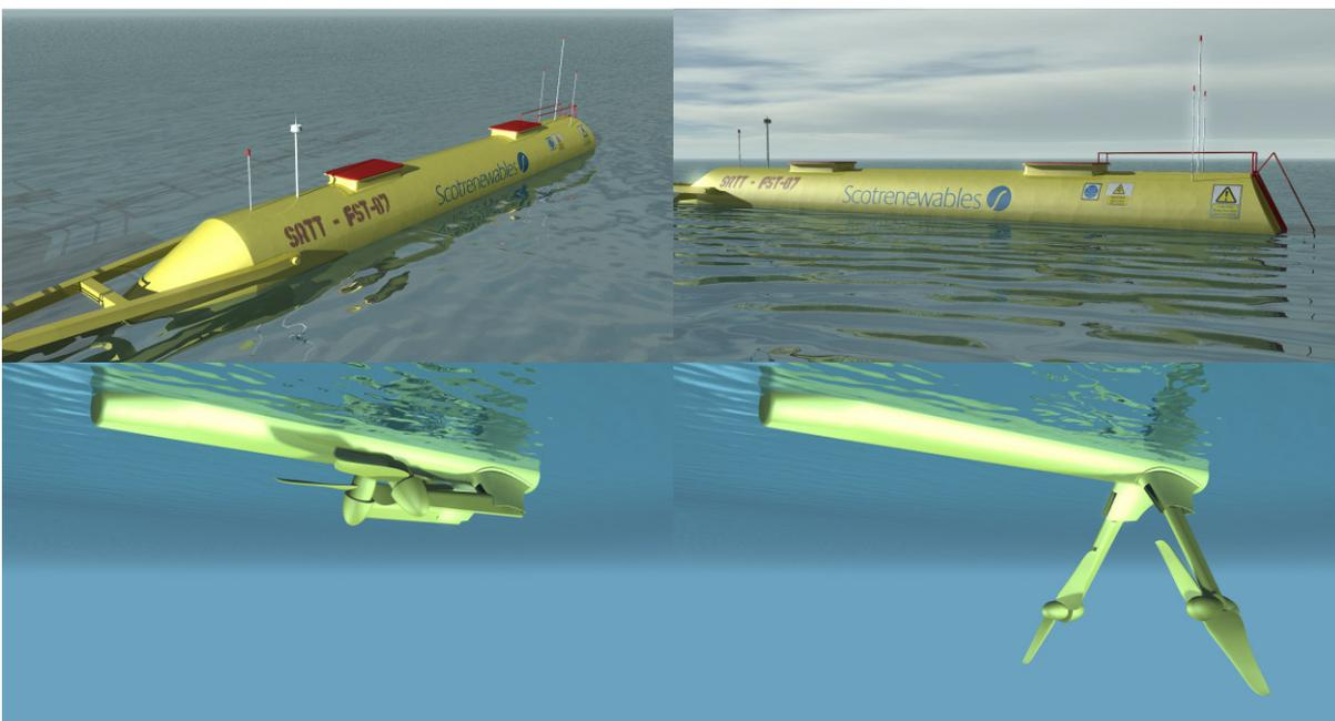
**Figure 1.1: SRTT Transport and Operation Configurations**
