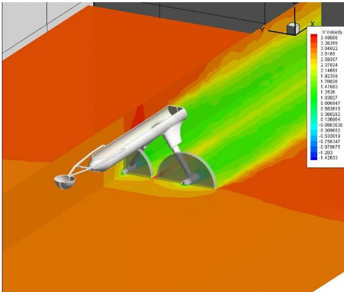
**Figure 2.7: Velocity field surrounding the SRTT**
