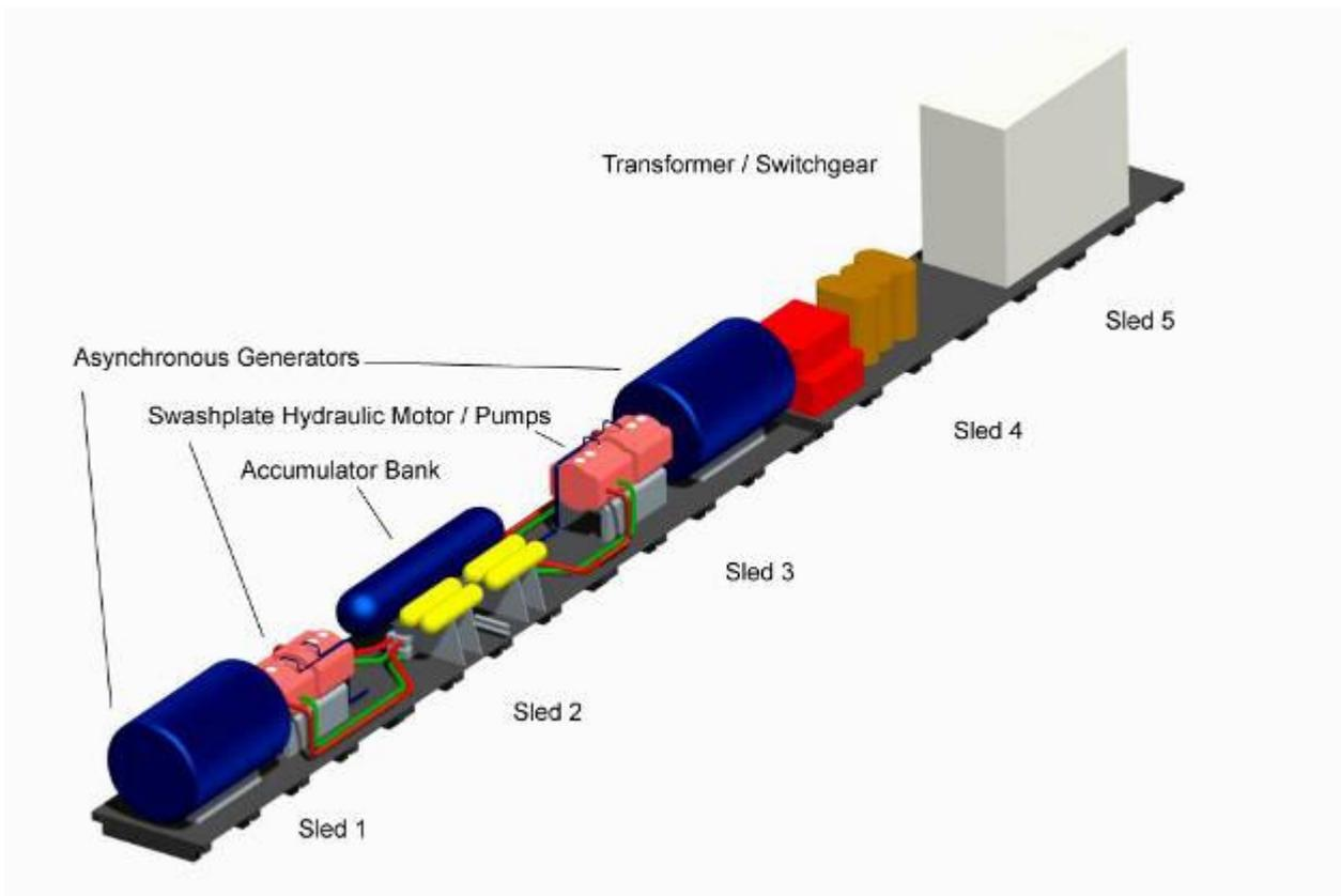
**Figure 2.4: SRTT Internal Component Modular Sled Assembly**
