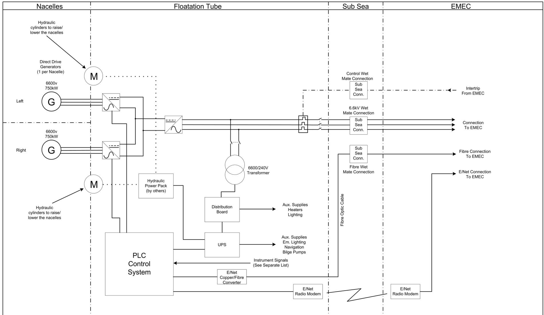
Figure 4.1: System Outline Option 1 – Electrical Direct Drive
