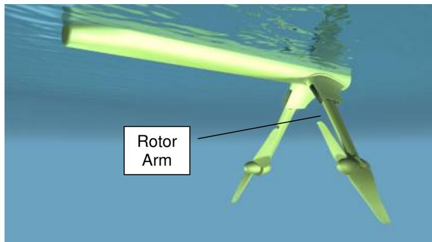
**Figure 2.9: SRTT Rotor Arm**
