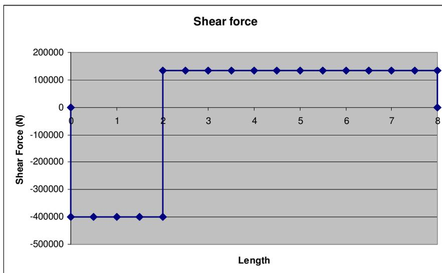
**Figure 2.12: Shear Force Diagram**
