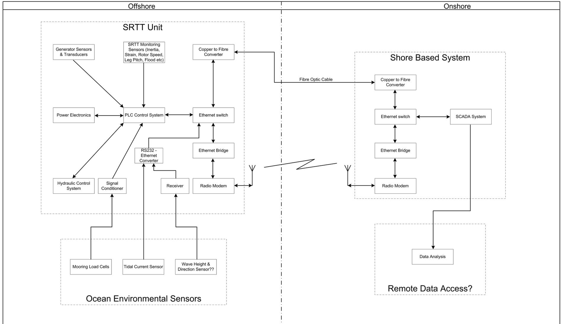
**Figure 4.4: Instrumentation and Control System Architecture**
