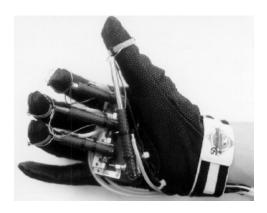
One type of data glove has a web of fiber optic cables along its back. Changes in the amount of light transmitted to the computer by the cables signal how the joints of your fingers are bent. Once the data glove has been calibrated to your hand, your gestures trigger pre-programmed commands.
