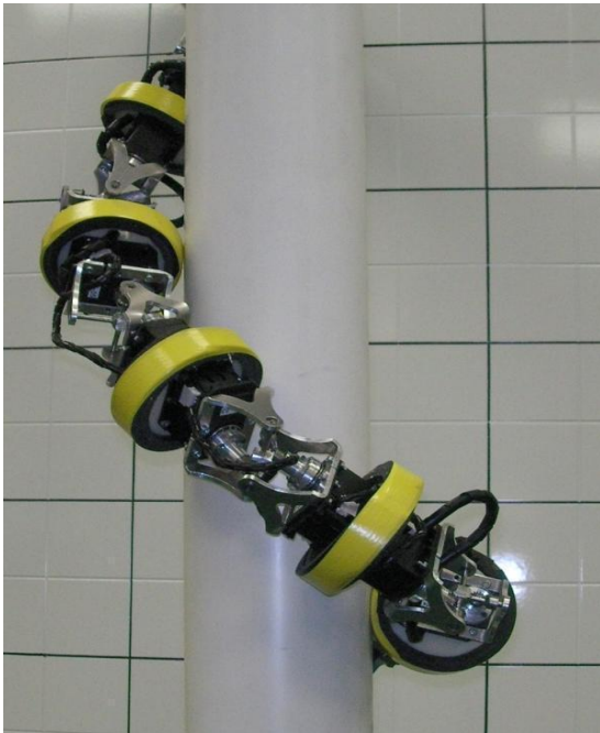
Fig: CIRCA – A Snake like robot Climbing on a Pillar
