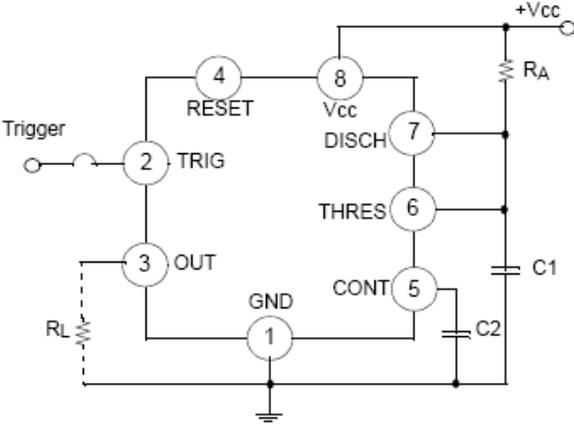
Here the popular 555 timing IC, is wired as a mono stable. The timing period is precise and equivalent to:-
