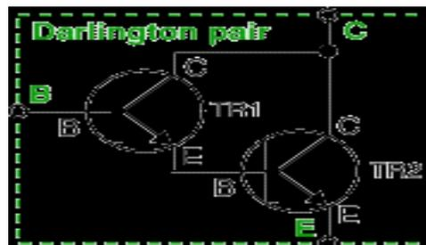
A darlington pair behaves as a single transistor with current gain equal to product of current gain of two transistors
