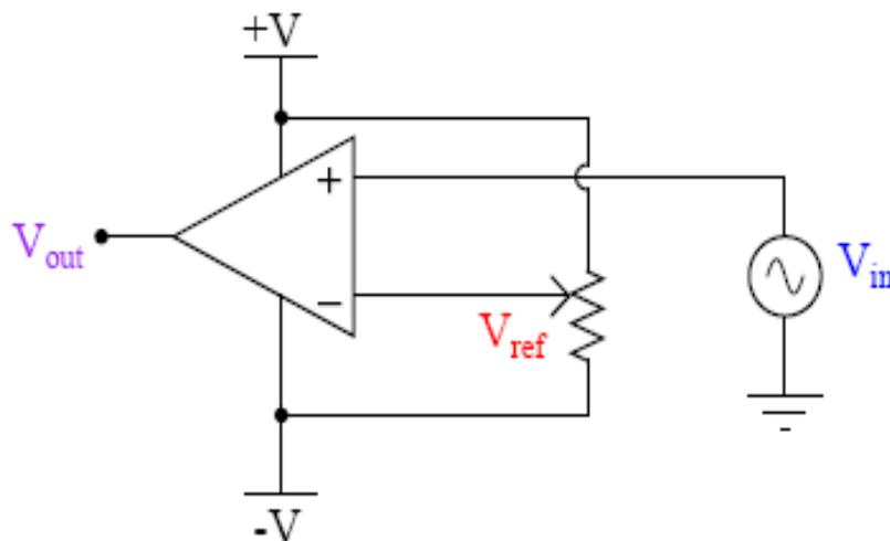
$V_{out}$  is high for  $V_{in}$  greater than  $V_{ref}$  and is low for  $V_{in}$  less than  $V_{ref}$ .
