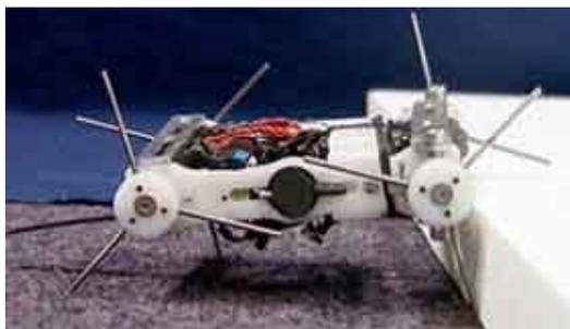
The robot pictured above is Whegs 1. It is 20 inches long, and utilizes three-spoke wheel-legs and one drive motor. It can climb obstacles of heights up to 1.5x the wheelleg radius, and the robot can move up to a speed of 3 body lengths/second (5.5km/hr).
