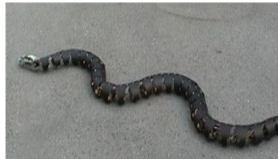
S5 represents a refinement of the S3 design. Parts were created using a numerically controlled milling machine. This allowed for much more accuracy, and a smaller cross-section. Almost doubling the number of segments allowed a robot that begins to resemble the length-to-width ratio of chubby real snakes. As the snake grows in size, the design starts to place heavier requirements on the wiring and control capability.
