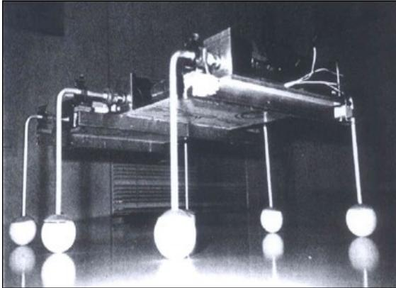
During the swing phase of walking, its feet rapidly rotate to return to the stance phase, when the feet rotate much more slowly. It uses a total of 6 motors and spoke-like legs to move.
