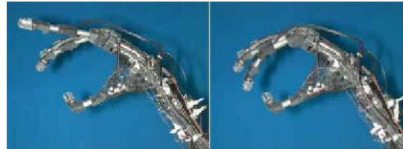
Given fig. demonstrates the flexibility of EAP actuators.
