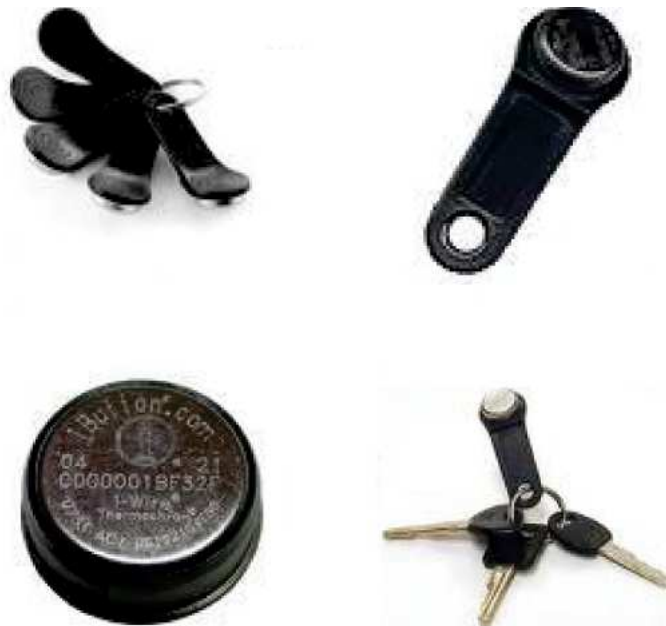
Figure 4.3: Different types of iButtons available in the market[1]
