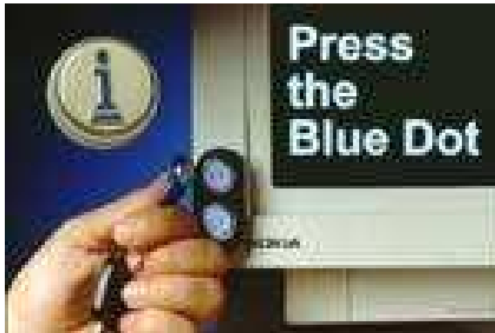
Figure 6.1: Application of java ring for getting account balance of a user through internet[1]
