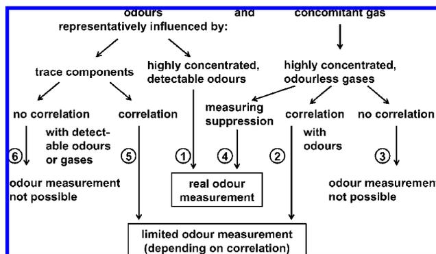
**Figure 1.** Schematic demonstrating the possible conditions for a reliable odor measurement. For target analytes not causing the human odor impression but which are of interest for other reasons the same flow diagram is applicable. Therefore, analytical background knowledge is important for the best adaptation of the system. Reprinted with permission from ref 10. Copyright 2003 Springer-Verlag.
