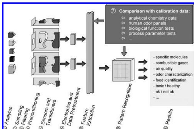
**Figure 2.** Schematic setup of a sensor system. Via sampling, filtering, and preconditioning the analytes are led to the sensing elements. These consist of a sensitive layer and a transducer to transform the chemical information into an electrical one. After the signal is recorded, data pretreatment, and feature extraction, pattern recognition evaluates the data using the calibration data. Reprinted from ref 11. Copyright 1998 American Chemical Society.
