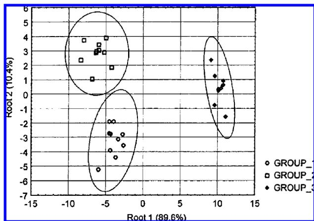
**Figure 15.** DFA of randomly generated data for a theoretical 24-sensor array. A total of 30 data points with a relative standard deviation of 7% were arranged into 3 groups of 10 data points. DFA discriminated them with a confidence interval (shown ellipses) of 95%. Reprinted with permission from ref 230. Copyright 2001 Elsevier.
