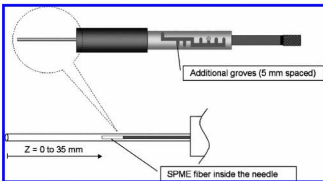
**Figure 12.** Schematic of an SPME fiber. To take a sample, the fiber is extended through the needle and exposed to the target analytes. After the volatiles have reached equilibrium between the fiber coating and the gaseous phase (or after a strongly defined time), the fiber is withdrawn into the needle. Desorption will take place in a heated inlet under a similar procedure. Reprinted with permission from ref 211. Copyright 2006 Elsevier.
