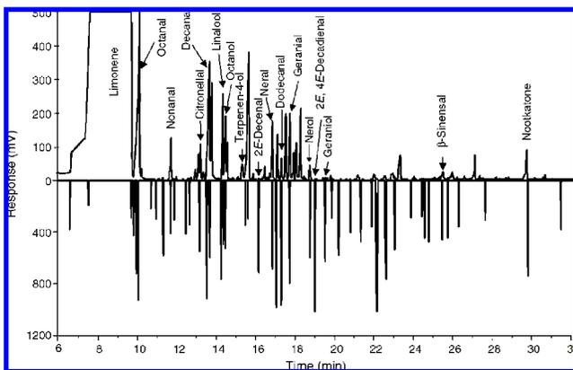
**Figure 6.** Comparison of a GC/FID chromatogram (top) with a time-intensity aromagram (bottom, inverted) of grapefruit oil. Some odorants have been identified by mass spectrometry. It is obvious that the human nose is sensitive to substances the flame ionization detector is not able to detect and vice versa. Reprinted with permission from ref 56. Copyright 2001 John Wiley & Sons, Limited.
