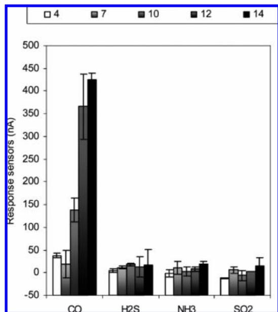
**Figure 10.** Response of the electrochemical gas sensors toward cod fillets during storage at 0.5 °C on days 4, 7, 10, 12, and 14. The CO sensor was most sensitive to changes during spoilage because of its sensitivity to alcohols, aldehydes, and esters (Figure 9). Although the trimethylamine concentration increased significantly at day 14, neither the NH<sub>3</sub> sensor nor the other ones contributed additional information. Reprinted from ref 100. Copyright 2005 American Chemical Society.
