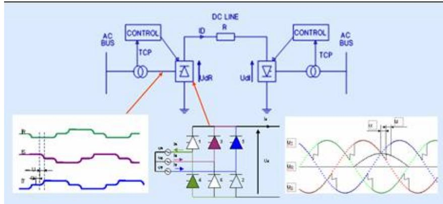
Fig. 10. Control of conventional HVDC transmission
