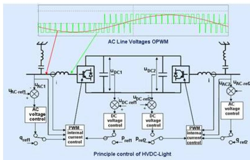
Fig. 11. Control of VSC-based HVDC transmission
