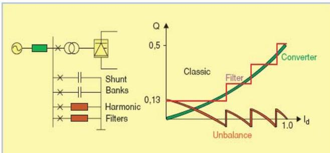
Fig. 8. Reactive power compensation for conventional HVDC
