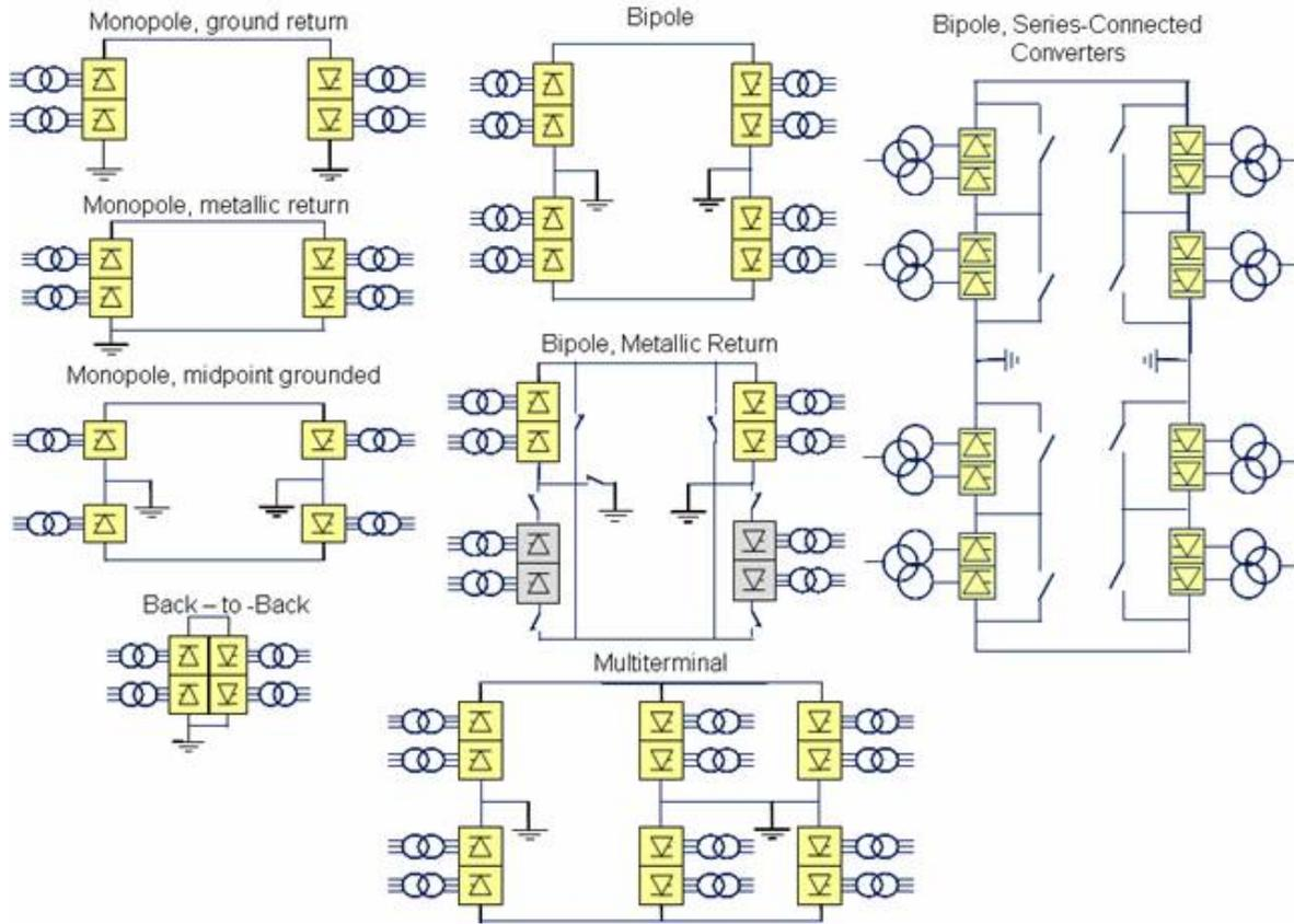
Fig. 3. HVDC configurations and operating modes
