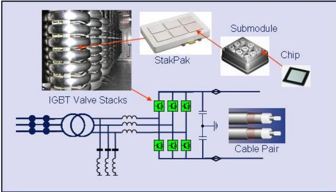
Fig. 7. HVDC IGBT valve arrangement
