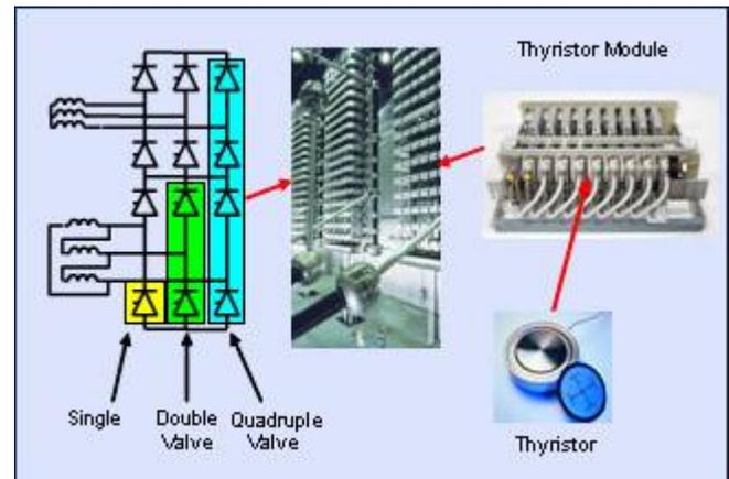
Fig. 6. HVDC thyristor valve arrangement
