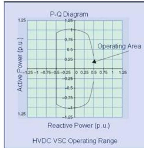
Fig. 9. Active - reactive power operating range for VSC based HVDC
