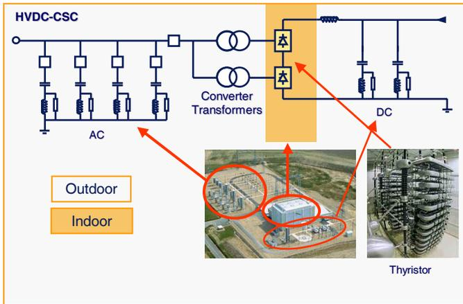
Fig. 4. Conventional HVDC with current source converters
