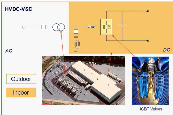
Fig. 5. HVDC with voltage source converters
