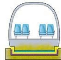
Electromagnets on the guideway levitate the car.
