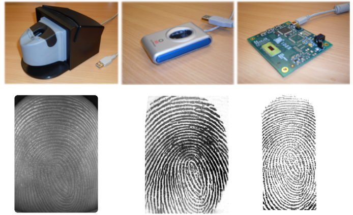
Fig. 1. Left: touchless optical sensor (TST BiRD3), Middle: optical sensor (DP U.4000), Right: capacitive line sensor (IDEX SmartFinger ® IX 10-4 ) and a fingerprint image from each database, at the same scale factor.
