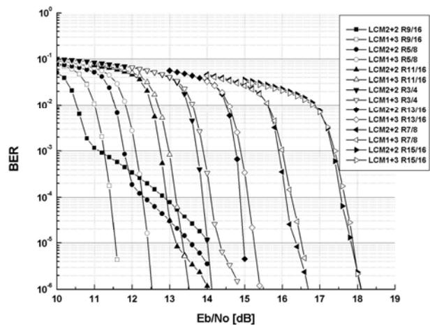
Fig. 6 Performance of LCM1+3 scheme versus LCM2+2 scheme (for various spectral efficiencies with 256-QAM in AWGN channel)
