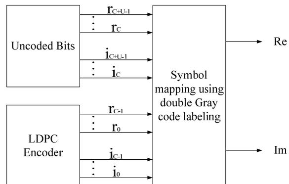
Fig. 2 LDPC coded modulation encoding and symbol mapping (for  $2^m$ -QAM, where  $U+C = m/2$ .)
