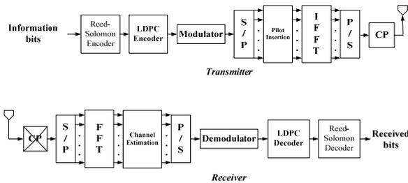
**Fig. 3 Reed-Solomon with LDPC-coded modulation (RS-LCM) WiMAX OFDM-256 PHYs**
