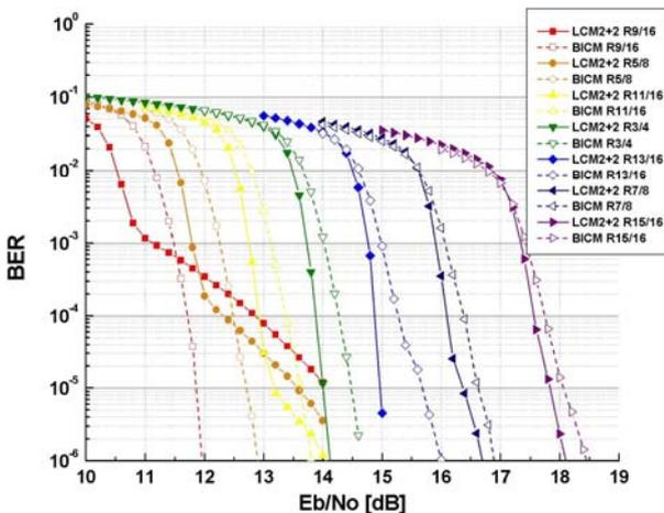
Fig. 4 BER Performance of LCM2+2 scheme versus BICM scheme (for various spectral efficiencies with 256-QAM in AWGN channel)
