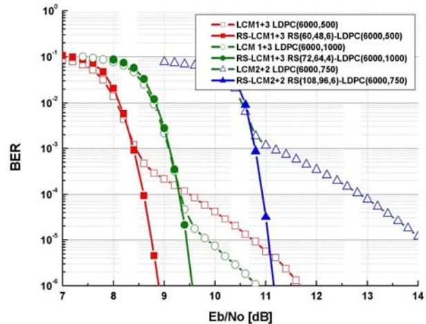
Fig. 7 Performance of RS-LCM versus LCM over AWGN channel with 256-QAM
