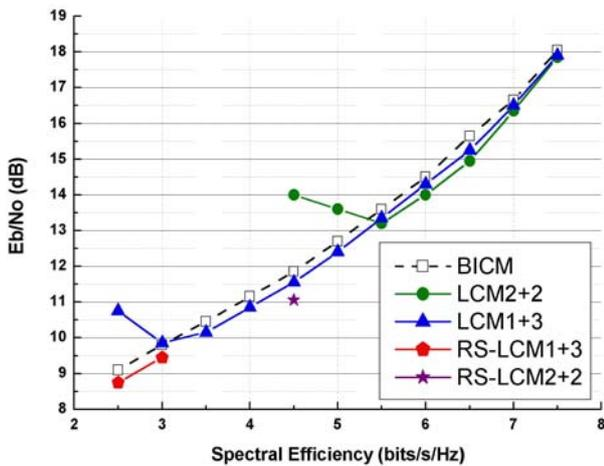
Fig. 8 Different LDPC coded modulation schemes comparison at BER  $10^{-5}$  over AWGN channel
