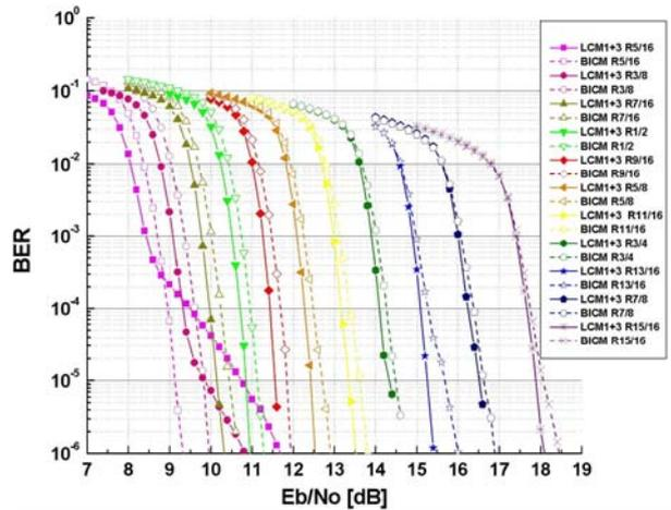
Fig. 5 BER Performance of LCM1+3 scheme versus BICM scheme (for various spectral efficiencies with 256-QAM in AWGN channel)
