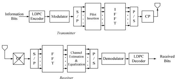
Fig. 1 Block diagram of WiMAX OFDM-256 PHYs
