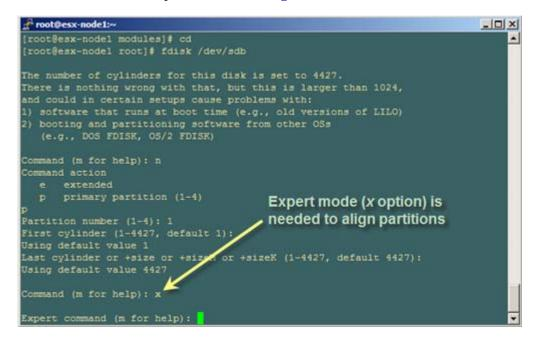
Figure 13 Using fdisk to create track-aligned partition
