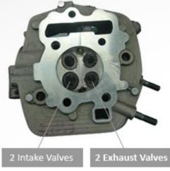
and longer at higher engine speeds when extra power is required.
