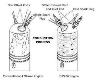
system on the Twin spark is a digital system with static spark advance and no moving parts subject to wear. It is mapped by the integrated digital electronic control box which also handles fuel injection and valve timing. It features two plugs per cylinder.
