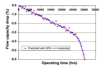
**Fig. 9.** Implanted compressor flow capacity degradation and predicted degradation with *GPA*.
