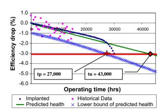
Fig. 10. Linear regression to scattered data of compressor efficiency at 15,000 h.
