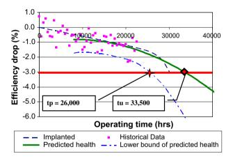
Fig. 14. Quadratic regression to scattered data of compressor efficiency at 22,500 h.
