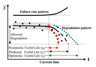
Fig. 1. Degradation and prognostic model.
