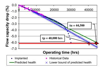
Fig. 11. Linear regression to scattered data of compressor flow capacity at 15,000 h.
