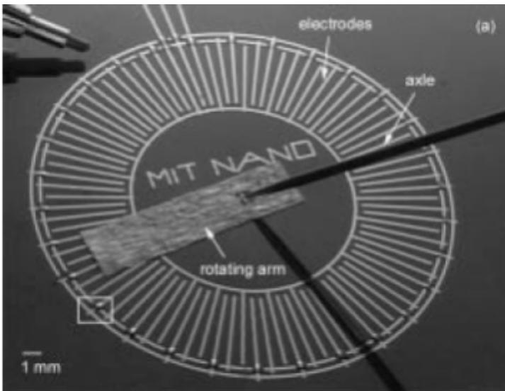
Ink-Jet printed electrostatic induction motor
