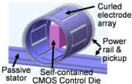
The millimeter scale catom consists of a tube and a High voltage CMOS die attached inside the tube. The tubes are fabricated as double-layer planar structures in 2D using standard photolithography. The difference in thermal stress created in the layers during the fabrication process causes the 2D structures to bend into a 3D tube upon release from the substrate. The tubes have electrodes for power transfer and actuation on the perimeter.
