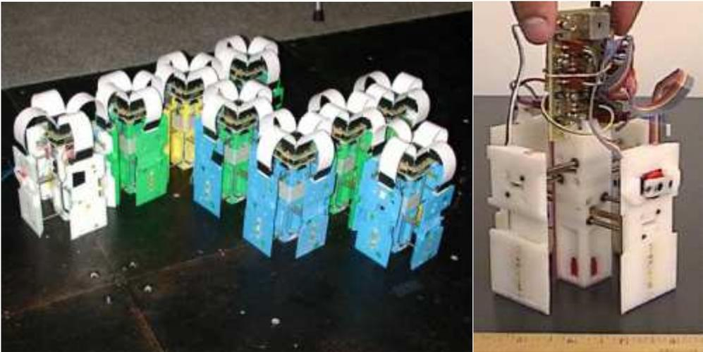
Vona and Rus's Crystalline robot (left) has unit-compressible modules (right) that can change size by a factor of two and latch for reconfiguration and amoeba-like mobility.
