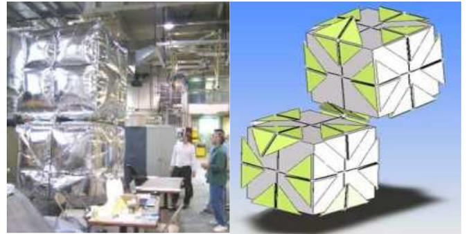
with a modular robot designed for self-construction of macro-scale structures.
