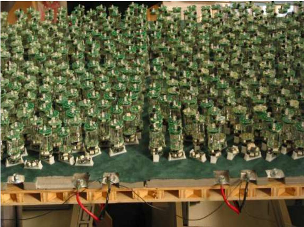
The centimeter-scale paintable display prototype.
