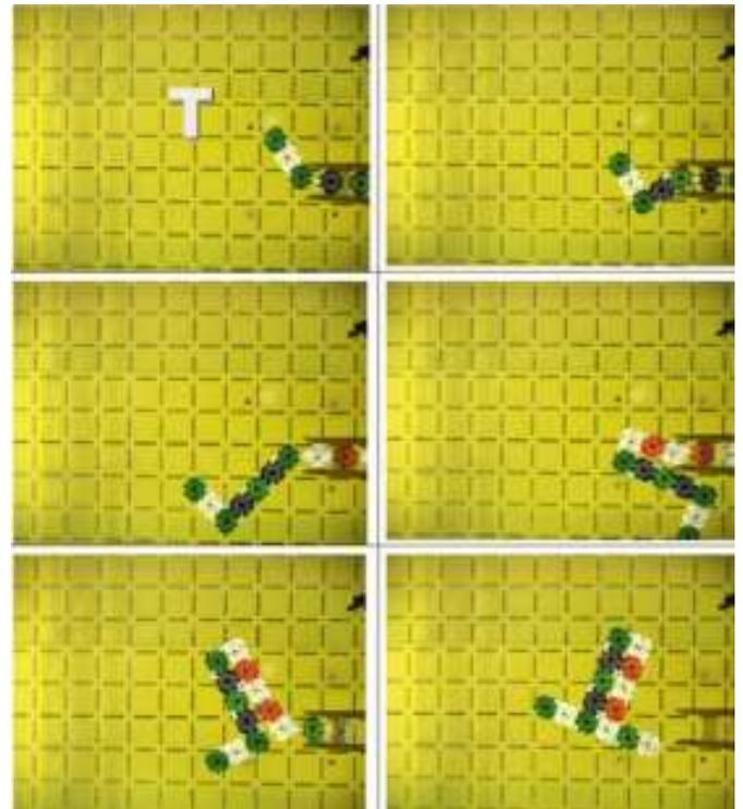
Digital fabrication of the letter "T," by folding a sequence of magnetic tiles that code for the structure
