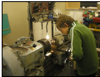
I am using the lathe to machine the spinning disc
