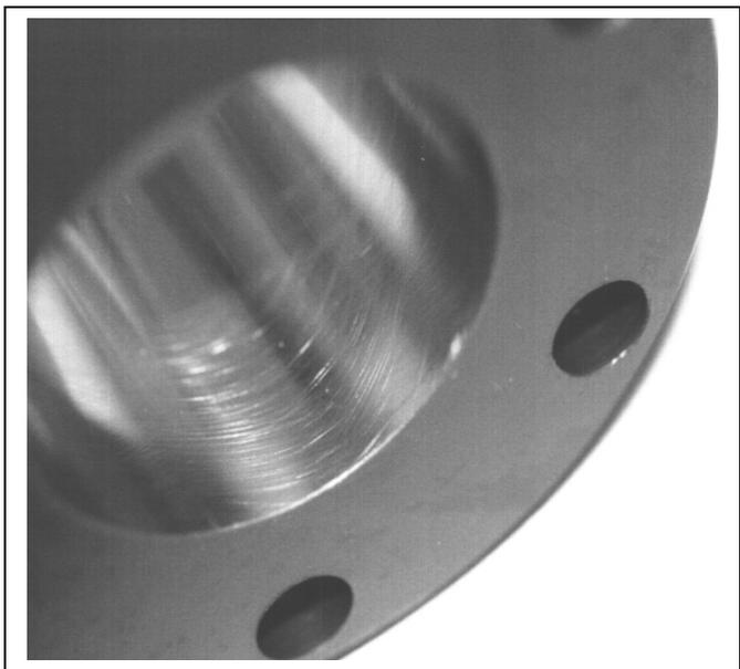
*Figure 2. M2 tool steel sleeve bore after lubricated test with silicon nitride ball. Original hone marks are still visible, and no wear is observed.*
