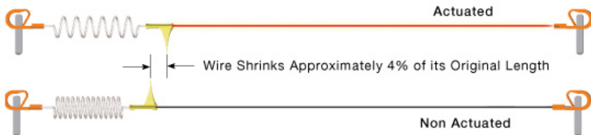
Shape Memory Alloy Wire Motion Principle
