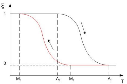
In this figure,  $\xi(T)$  represents the martensite fraction. The difference between the heating transition and the cooling transition gives rise to hysteresis where some of the mechanical energy is lost in the process. The shape of the curve depends on the material properties of the shape-memory alloy, such as the alloying.<sup>[2]</sup> and work hardening.<sup>[3]</sup>
