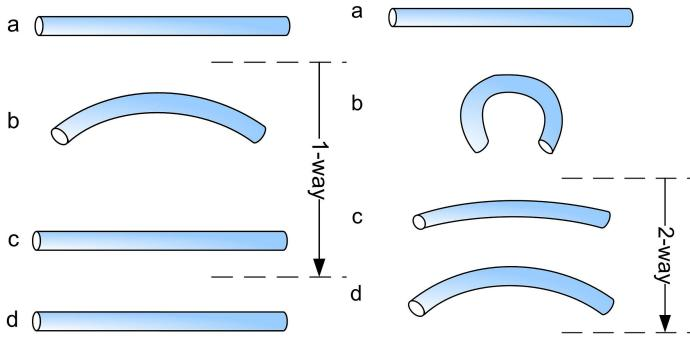
The procedures are very similar: starting from martensite (a), adding a reversible deformation for the one-way effect or severe deformation with an irreversible amount for the two-way (b), heating the sample (c) and cooling it again (d).
