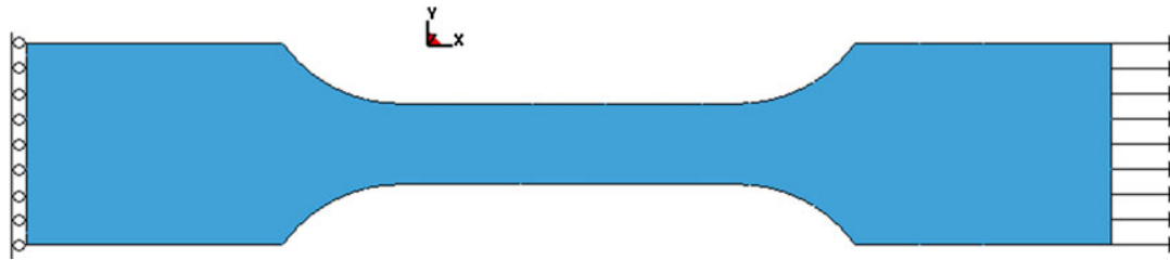
Fig. 3 Schematic of isothermal uniaxial tension loading
