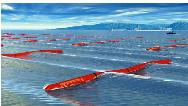
Fig. 1 Attenuator device: Pelamis wave farm [17]
