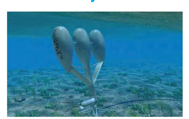
The bioWAVE oscillating wave surge converter system is based on the swaying motion of sea plants in the presence of ocean waves. In extreme wave conditions, the device automatically ceases operation and assumes a safe position lying flat against the seabed. This eliminates exposure to extreme forces, allowing for light-weight designs.
