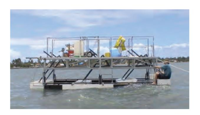
The PerpetuWave captures wave energy through a series of articulated arms mounted on the bottom or a larger floating craft. Each of the articulated arms has a float mounted on the end, as waves pass under the larger craft the articulated arms are forced to move up and down with the waves. The mechanical energy in the arms is converted on board into electricity.
