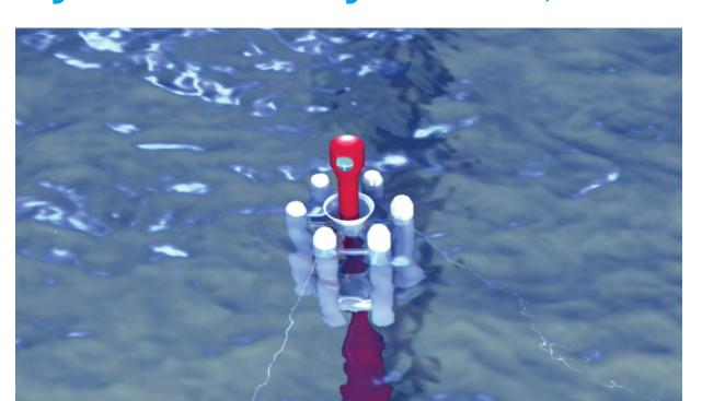
The SyncWave Power Resonator device creates power by capturing the motion differential (phase lag) between two dissimilar float structures. Power is captured by a hydraulic power take-off, driving a permanent magnet DC generator. DC power from several SyncWave units in a wave farm will be collected and converted to AC power in a seabed mounted collector hub.
