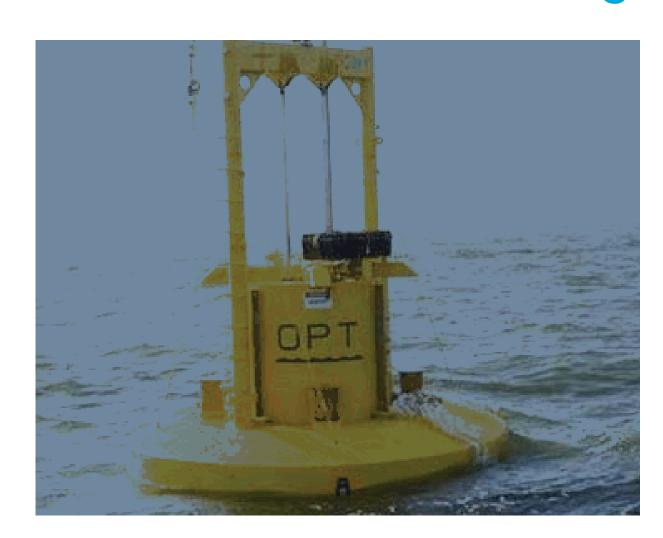
The Ocean Power Technologies wave power station consists of an array of PowerBuoys typically located two to three miles offshore. A PowerBuoy is a loosely moored buoy-like structure (point absorber device) that rises and falls on the waves. The resulting mechanical energy is converted into electrical energy by the use of a power take-off device, an electrical generator and an electronic control system, all of which are sealed inside the PowerBuoy.
