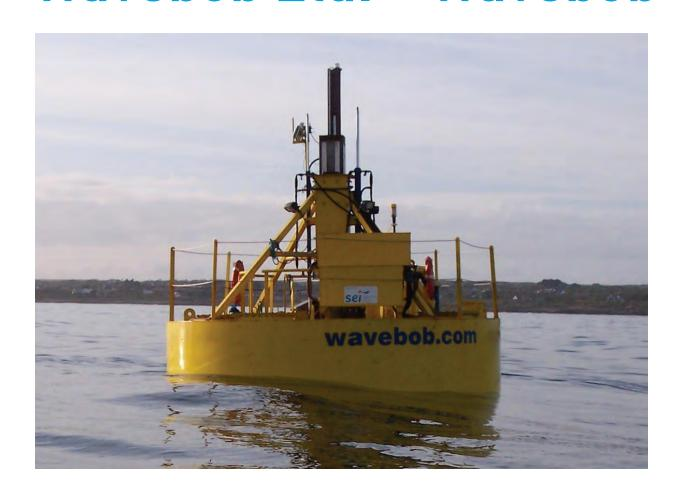
The Wavebob WEC can be moored and maintained in large multi-megawatt arrays offshore. Wavebob is a free floating, self-reacting, axi-symmetric point absorber. This is tuned to the incident wave action using a system to change the device's natural resonance frequency without changing the float's draught.
