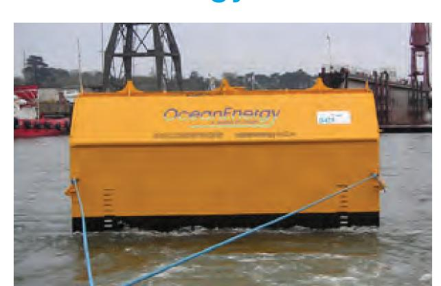
The OEBuoy is a floating, oscillating water column (OWC) that uses wave energy to compress air in a plenum chamber and pump it through an air turbine system. The mouth of the OWC faces away from the wave direction, resulting in high energy efficiencies at the operating point due to the motions of the float system relative to the waves.
