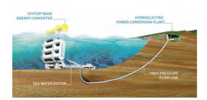
The Oyster is uniquely designed to harness wave energy in a near-shore environment. It is composed primarily of a simple mechanical hinged flap connected to the seabed at a depth of about 10 meters and is gravity moored. Each passing wave moves the flap, driving hydraulic pistons to deliver high pressure water via a pipeline to an onshore electrical turbine.
