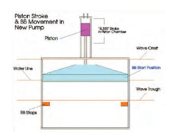
The SEADOG uses a differential in float capacity to captures wave energy. As waves pass through the device it causes the center float block to move up and down relative to the exterior. This motion drives a piston which pumps sea water. The SEADOG is being developed for both seawater desalination systems and hydroelectric energy generation.
