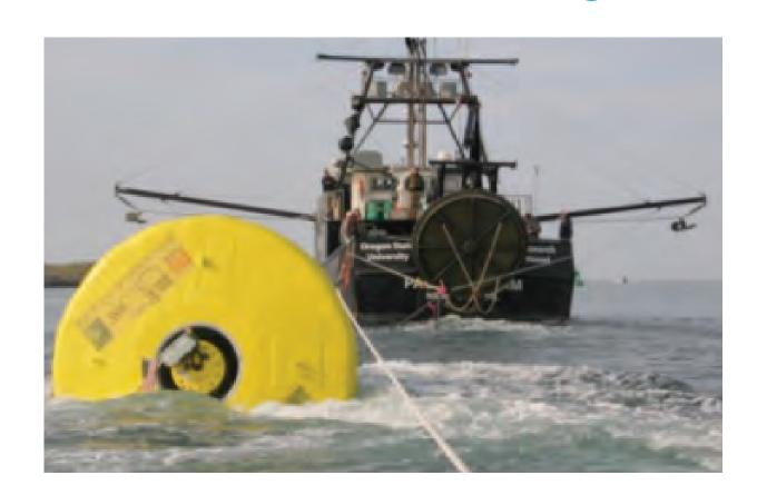
Columbia Technologies is developing a "Point Absorber" wave energy capture device. Moored two to three miles off the coast, the point absorbers use the undulation of the waves to move an outer floating sheath of magnets around an inner copper coil of wire. As the magnets move around the copper coil, the changing position of the magnetic field causes voltage to be generated. The electricity generated by the device runs via cable to shore.
