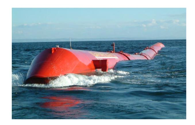
The Pelamis wave energy converter is a free floating, hinged attenuator device. This device consists of four tubular sections connected by three hinged modules, which move relative to each other. This motion is converted to power by means of a hydraulic power conversion system in each of three power conversion modules. The Pelamis is slack-moored with a compliant mooring configuration that both points the device into the waves and enhances survivability.
