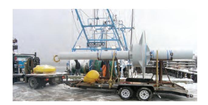
Resolute is a point absorber wave energy capture device and is still in the developmental stage. The final design of the device has yet to be determined. The depth at which it will operate and the means by which it will be mounted to the sea floor are also still unknown.
