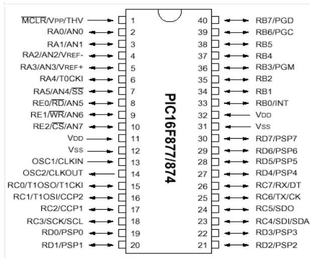
The PIC micro controller board consists of circuits necessary to operate a micro controller with PC interface. To have a PC interface for a heart beat rate-monitoring system we have used a PIC micro controller IC PIC16F877.
