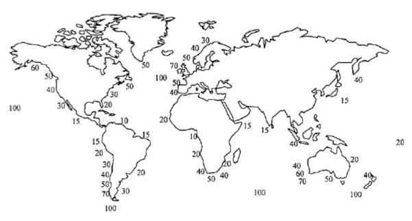
Fig. 1 Approximate global distribution of wave power levels (kW/m of wave front)
