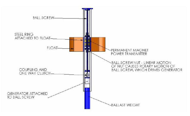
Fig. 12 Contact-less Force Transmission System [26]
