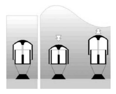
Fig. 7 Below Surface Point Absorber [4]
