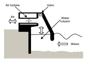
Fig. 5 Oscillating Water Column Device [9]
