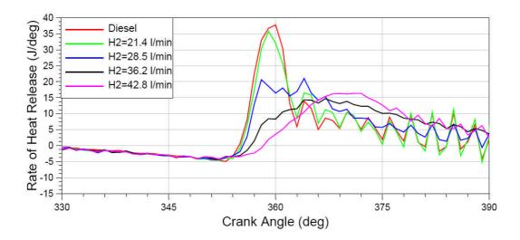
Figure 7: Rate of heat release at 2000 rpm, 5 Nm
