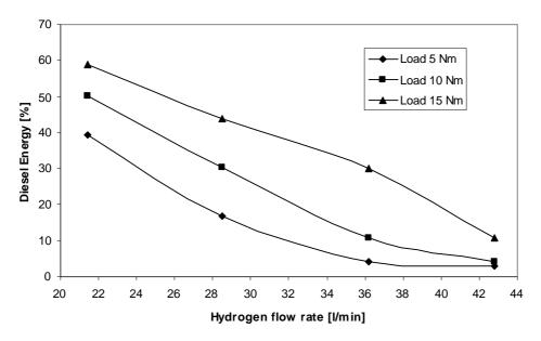
Figure 2: Diesel energy replacement by hydrogen
