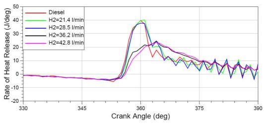
Figure 9: Rate of heat release at 2000 rpm, 10 Nm
