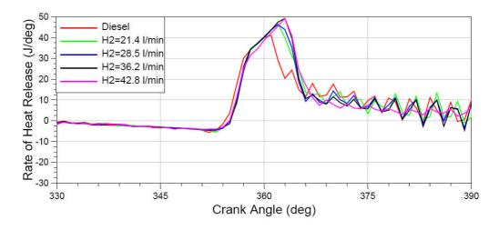
Figure 11: Rate of heat release at 2000 rpm, 15 Nm
