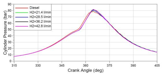
Figure 10: Cylinder pressure at 2000 rpm, 15 Nm
