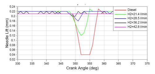
Figure 3: Needle lift at 2000 rpm, 5 Nm
