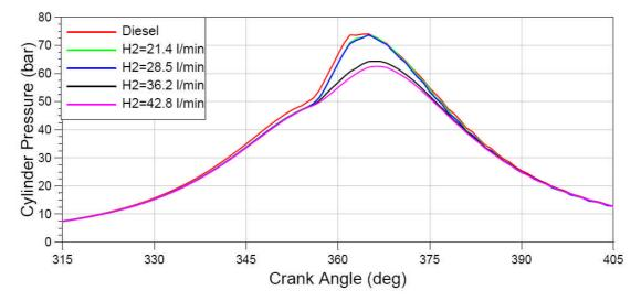
Figure 8: Cylinder pressure at 2000 rpm, 10 Nm
