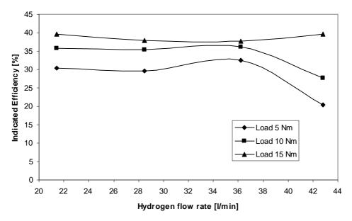
Figure 5: Variation of indicated efficiency with hydrogen enrichment and load
