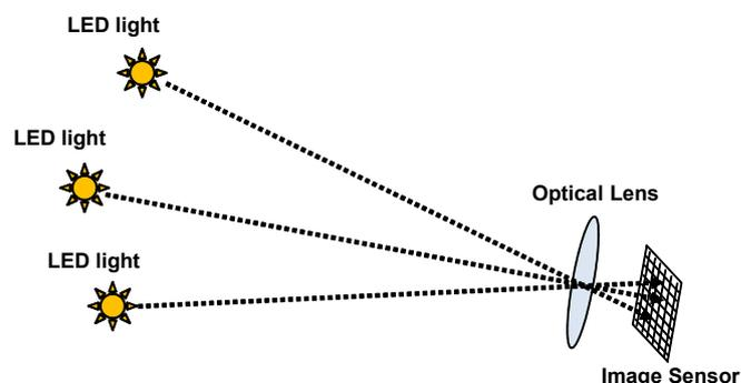
**Figure 12.** Concept of Visible Light Communication using Image Sensors as Receivers
