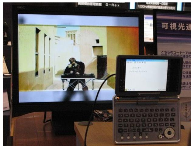
**Figure 6.** Visible Light Communication to send Information using LED Backlight of LCD Display
