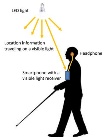
**Figure 8.** Indoor Navigation System for the Visually Impaired using Visible Light Communication
