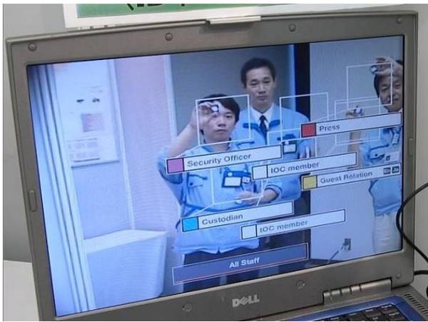
**Figure 13.** Application Example of Visible Light Communication using Image Sensors as Receivers
