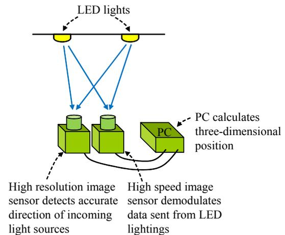
**Figure 15.** Robot Control System using Visible Light Communication
