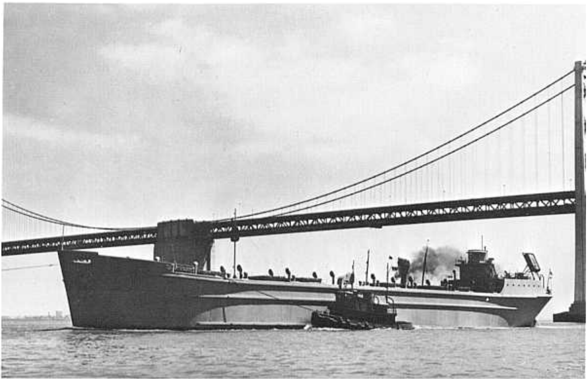
World War II concrete ship passing under San Francisco-Oakland Bay Bridge, San Francisco. Both ship and bridge made extensive use of structural lightweight concrete.
