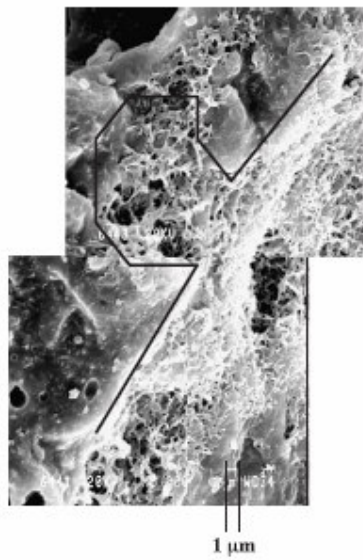
Figure 3.14. Porous Aggregate as Interlocking sites for HCP at the IZ (x5000) [18]
