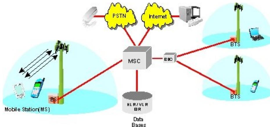
Global System for Mobile Communication - GSM System Diagram
