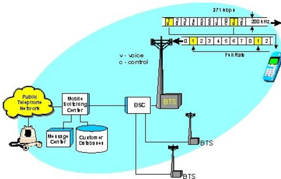
GSM Radio Channel Structure Diagram
