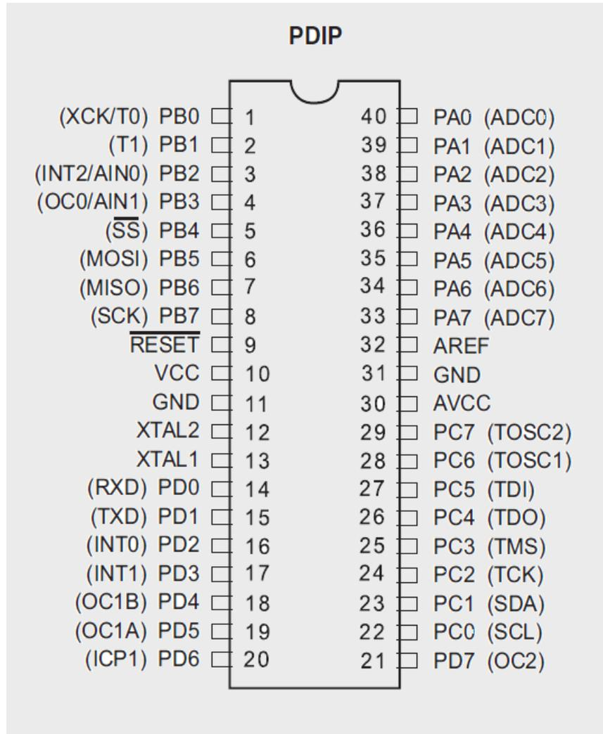
Fig 3.1: Pin diagram of ATmega16
