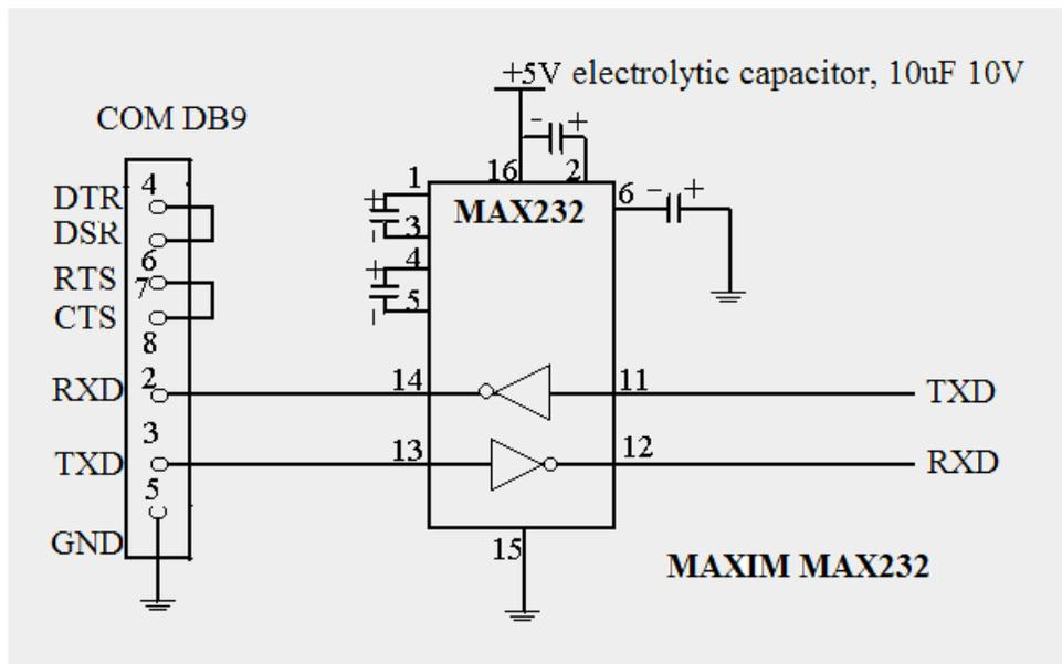
Fig 3.2: Connection between MAX232 and DB9 Connector.
