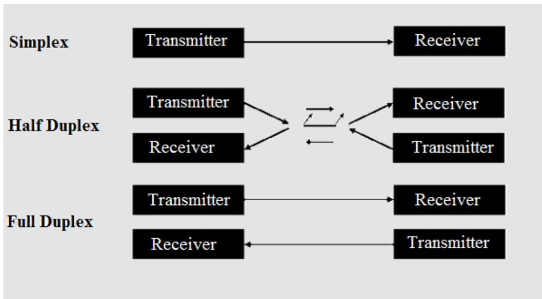
Fig 2.3: Diagrammatic Simplex & Duplex Transmission
