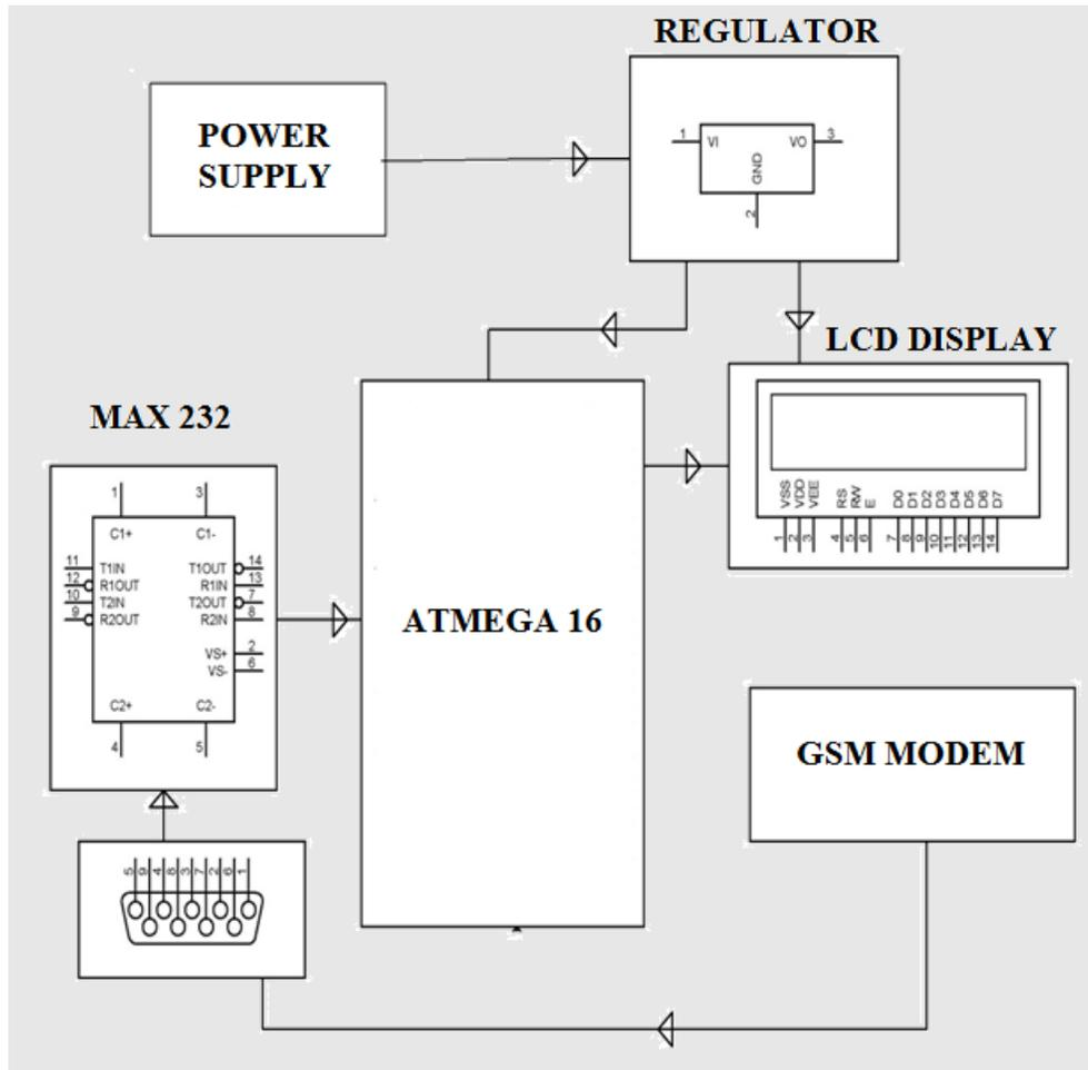
Fig 4.1 Circuit Schematic
