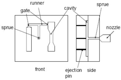
Mold (Tool and/or Mold) is the common term used to describe the production tooling used to produce plastic parts in molding.
