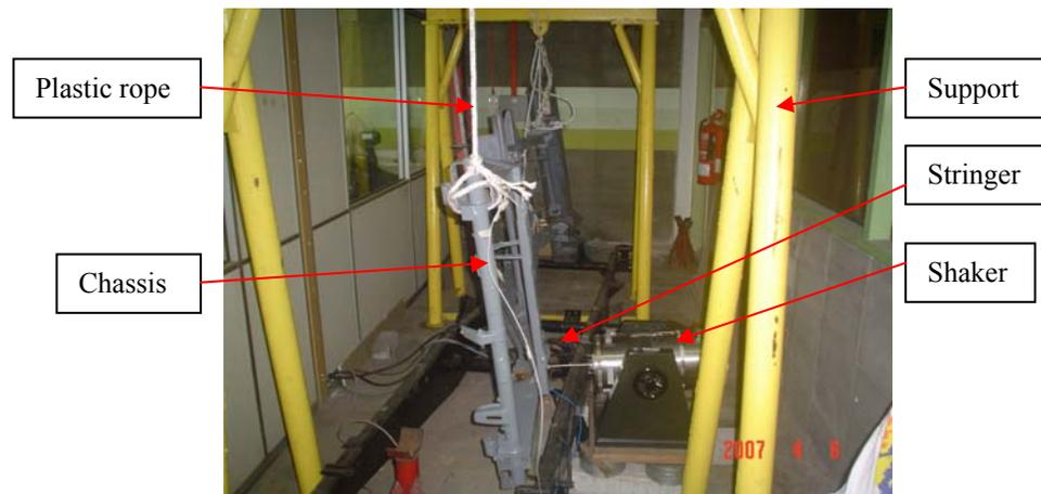
Figure 5.3: Shaker Test Set-up
