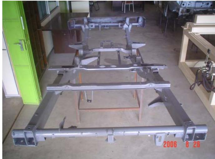
Figure3.1: Parallel ladder type frame
