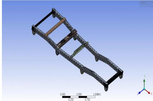
Figure 6.1: Truck chassis model meshed with tetrahedral -10 elements
