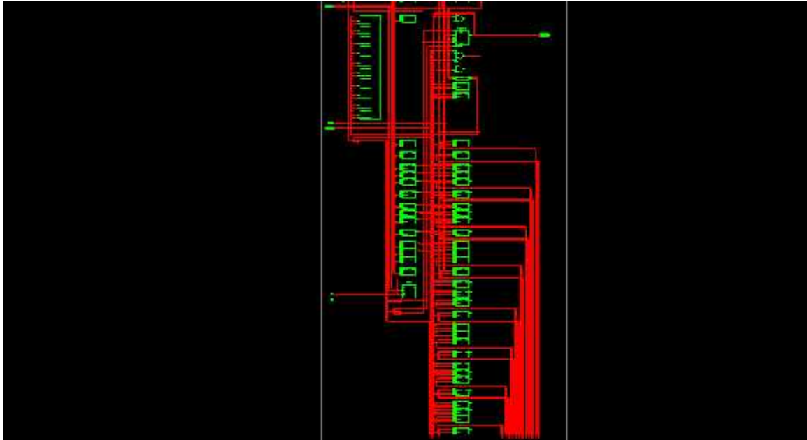
Fig 6.6: Register Transfer Logic for Barrel shifter
