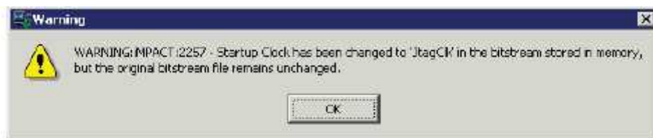
Figure 22 : iMPACT Issues a Warning if the StartUp Clock Was Not CCLK
