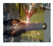
Cutting of various metallic materials such as alloy and structural steels, bronze, titanium.
