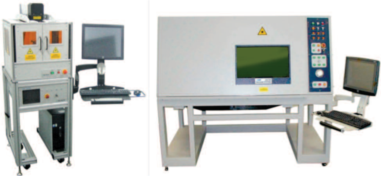
Figure 19. Class 1 enclosures for laser marker cutting system and a gas-assist fusion cutting system
