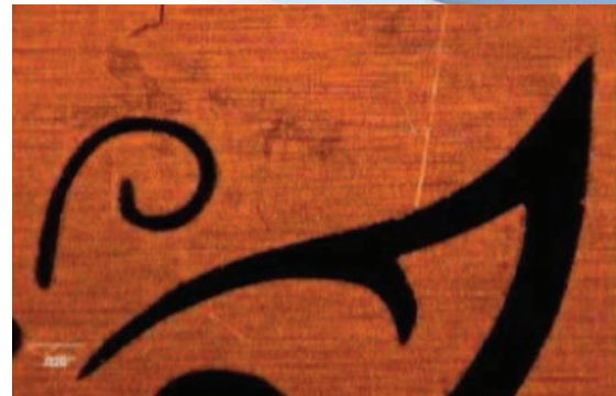
Figure 11. 0.02" thick copper sheet. The XY galvo beam delivery optics completed a 1" x 1" complex cut pattern in about 30 seconds.
