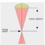
the distance between the focal point and the focussing optics. The focal point is positioned above, on or below the material surface according to the requirements of the material (See below: Focussing point depending the material). The power density heats up the material instantly, melting it and partially vapourizing it. The gas jet flowing through the cutting nozzle removes the molten mass away from the kerf.
