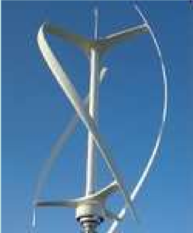
Helical wind turbine
