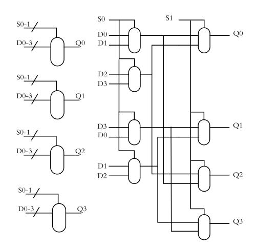
bit of the shifted result. But now, the remaining two bits requires only one multiplexor each, so the total number of multiplexors needed is eight instead of twelve. This advantage increases as the number of bits increases.
