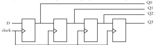
in this circuit every time the clock ticks all data moves one flip-flop to the right, with whatever data is currently on input D shifted into the first flip-flop. The disign you see is called a serial in, parallel out register because the data comes in one bit per clock tick, but can be read all at once on the outputs. Components like these are fundamental to serial buses of all kind, such as USB, because they convert a series of bits into a byte or a word.
