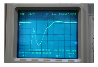
Figure 8. Opening of a plasma microwave barrier in microseconds.
