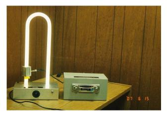
Figure 5. A Plasma Antennas connected to a Radio.
