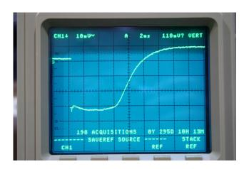
Figure 10. Attenuation E-field perpendicular to tubes.
