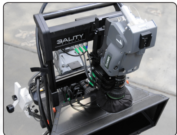
Figure 15 – LDK 8000 Elite Cameras on a new 3ality mirror system rig (cameras at 90° to each other).
