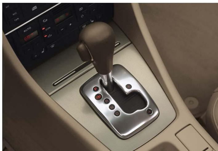
**Figure 8 :** Tiptronic transmission.
