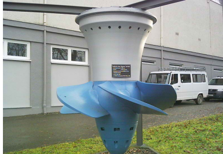
Figure 1.4: shows a photo of an actual Kaplan Turbine
