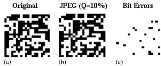
Fig. 5. (a) Fingerprint of original Lena image, (b) Fingerprint of compressed Lena image, (c) the difference between a and b showing bit errors in black (BER = 0.05).
