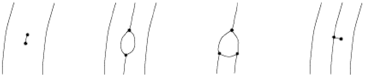
Figure 5.3: Examples of typical false minutiae structures : (a)Spur, (b)Hole, (c)Triangle, (d)Spike
