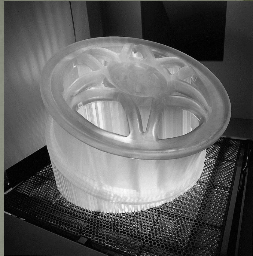
Figure A part produced by stereolithography (photo courtesy of 3D Systems, Inc.).
