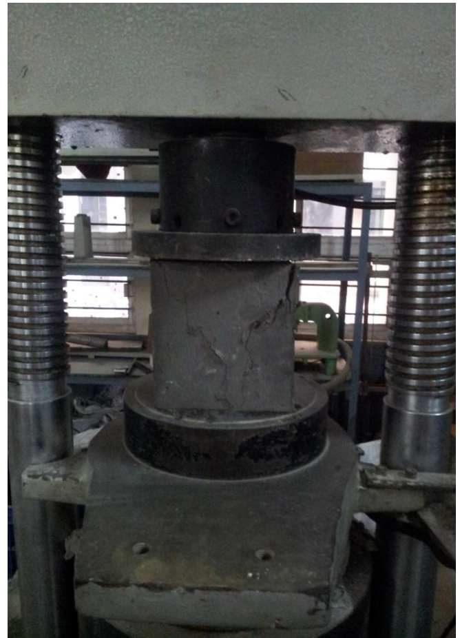
Fig -3: Concrete cube subjected to compression
