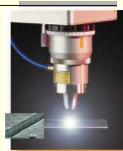
NdYAG pulsed laser for micromachining
