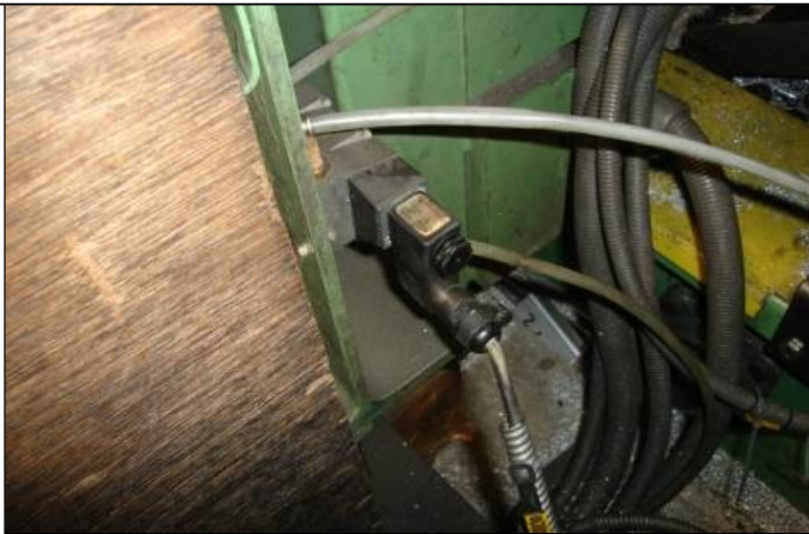
Solenoid fixing cap missing - replaced
